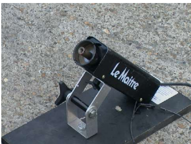
The solenoid unit mounted on a board
